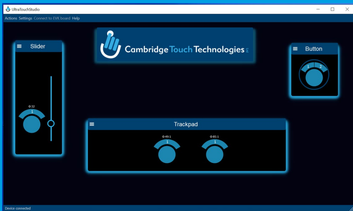
Screen shot of UltraTouch Studio in operation show simultaneous detection of fingers on the multi-force button, the force-based slider and the two-finger touch pad
