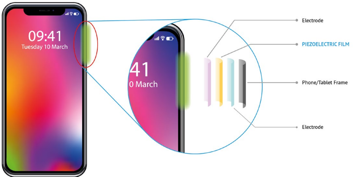
Figure 3 - Potential use case showing force sensing for button replacement
