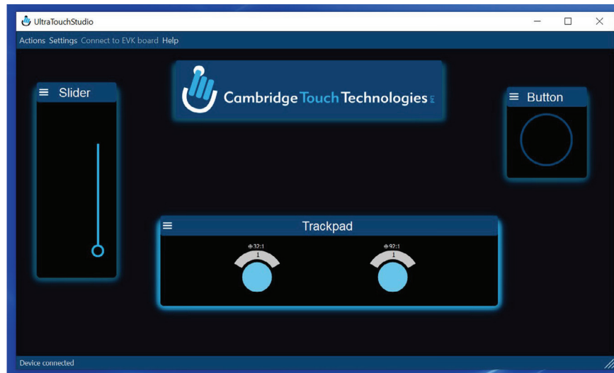
A two-finger touch event on the EVK touch pad displayed on the UltraTouch Studio application
