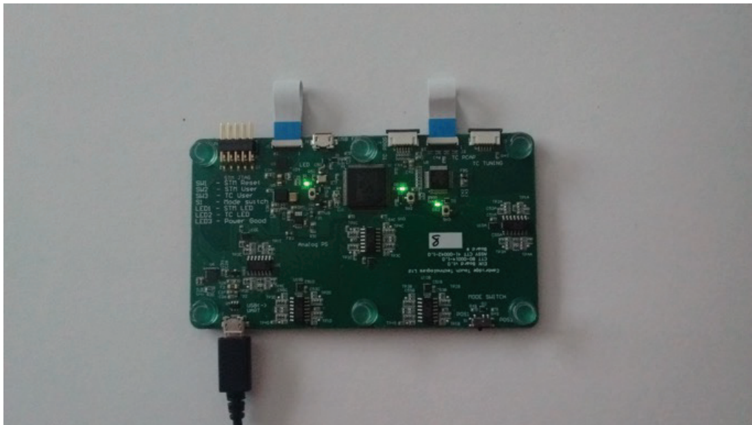
The underside of the EVK after successful power-up with LED DS3 – top left, constant green. LEDs DS1 and DS2 are not used in stand-alone mode and blink green.
