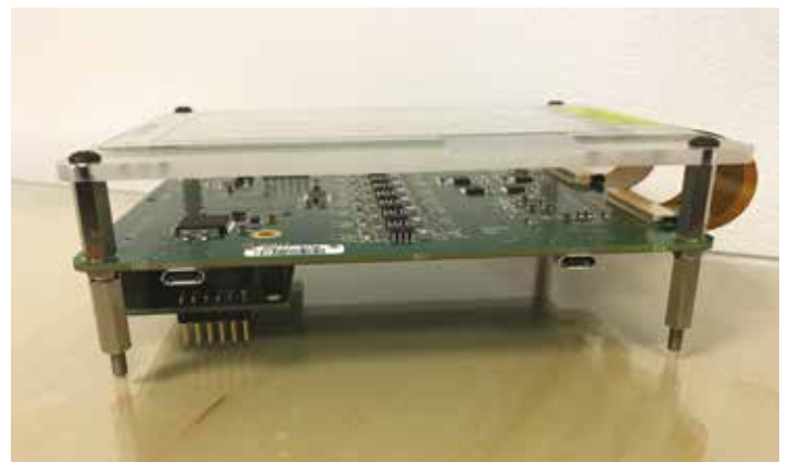
Assembled 4.3" force sensing touch platform. The thin glass force sensor is seen at the top, and built using a high volume manufacturing process for smartphone touch panels (Photo courtesy of Cambridge Touch Technologies)
